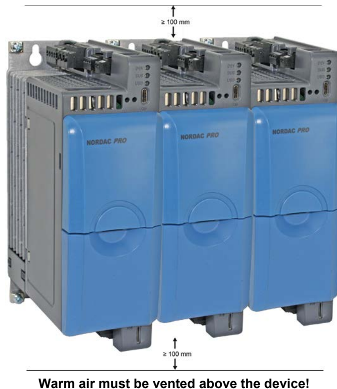
Figure 1: Installation spacings
