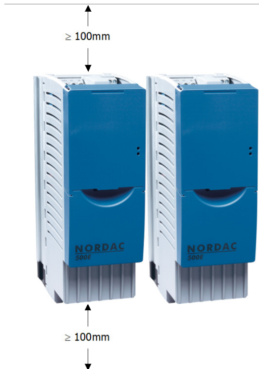
Fig. 1 Mounting distances for SK 5xxE
