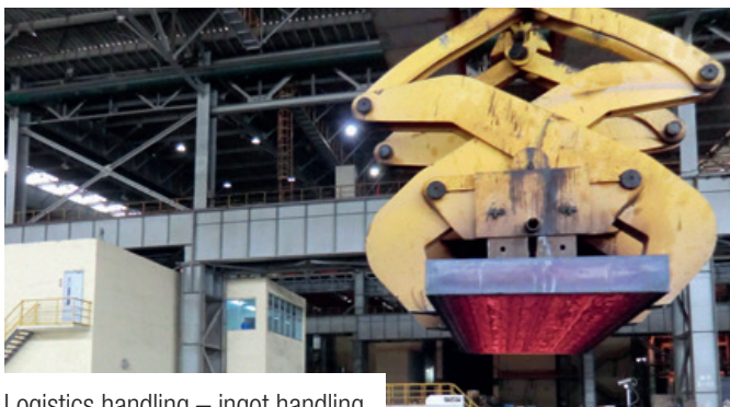
Logistics handling – ingot handling
