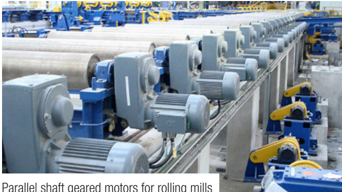
Parallel shaft geared motors for rolling mills
