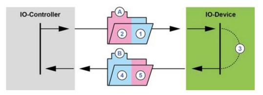
Figure 10: Structure of the application data area – Telegram traffic
